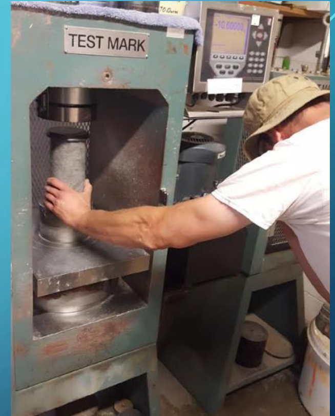
Figure 9 Crocket Breaking Cylinder [6]
