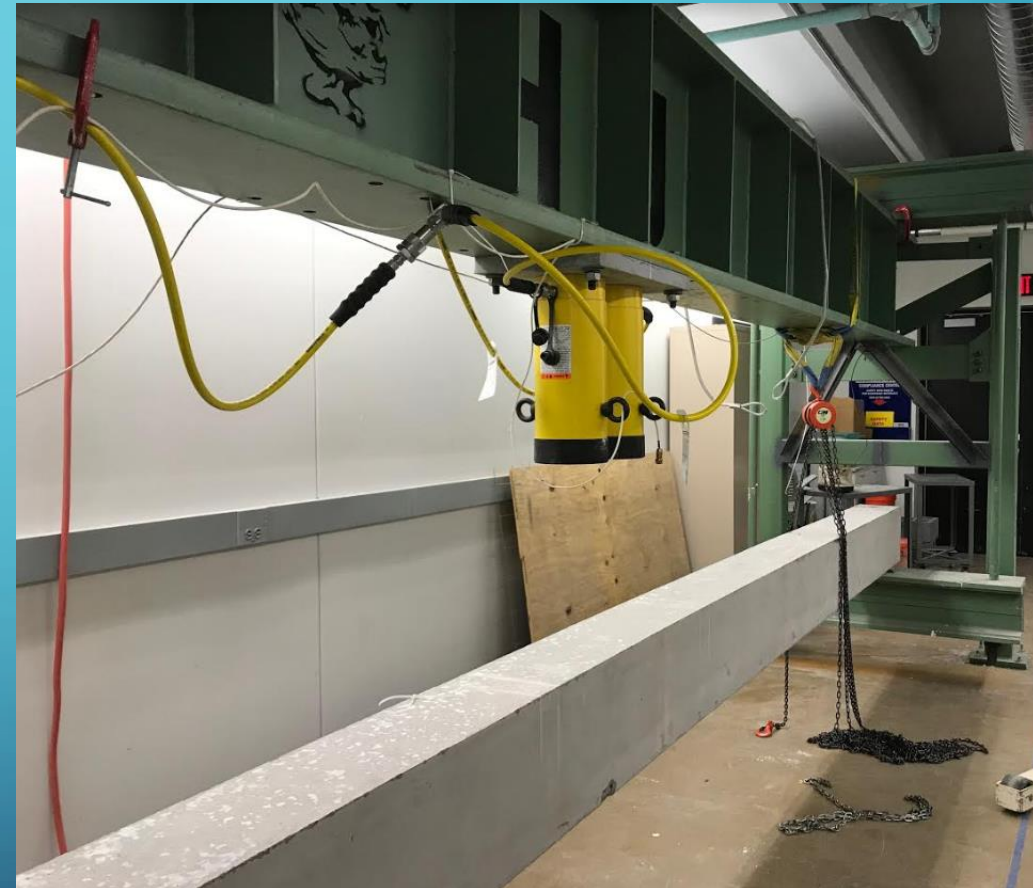
Figure 21 Current State of Beam Setup [2]
